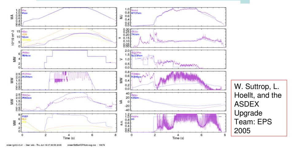
Figure 4: Comparison of predicted and measured waveforms of ASDEX Upgrade shot 18079
