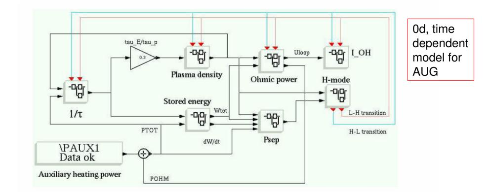
Figure 3: Scicos model for L- and H-mode plasma density, stored energy and ohmic transformer flux consumtion.
