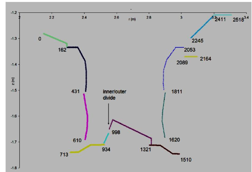
s-coordinate: distance along the surface of the divertor from the innermost point on the divertor to the outermost
