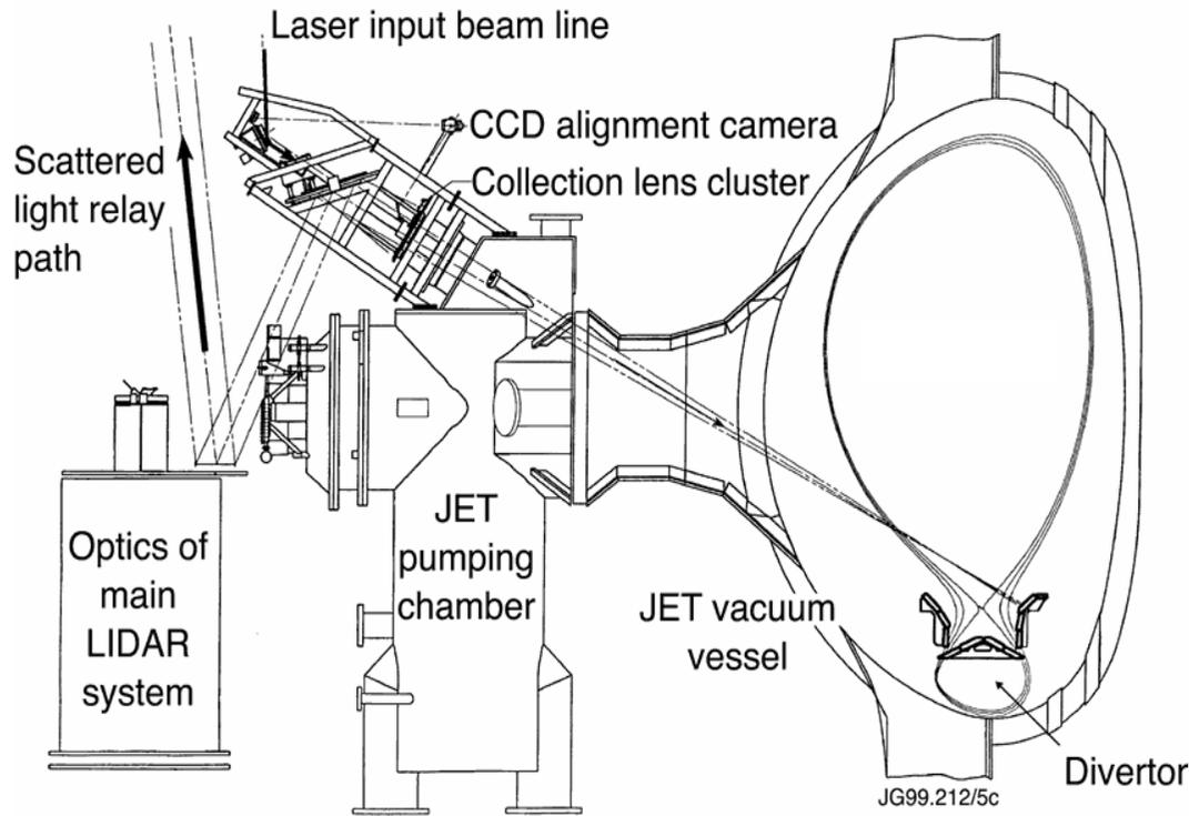
For Edge LIDAR because of flux surface mapping the spatial resolution is  $\sim 4 - 2$  cm, depending on plasma configuration (DOC-U)
