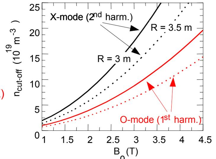
The cut-off density for the 2<sup>nd</sup> harmonic X-mode is twice that of the 1<sup>st</sup> harmonic O-mode
