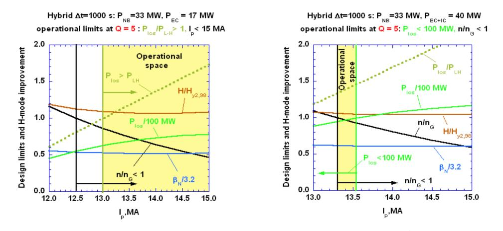
Hybrid scenarios with Q = 5,  $\Delta t$ = 1000 s, P<sub>fus</sub>= 250-365 MW (P<sub>aux</sub>= 50-73 MW) are possible for H ~1-1.1, P<sub>los</sub>/P<sub>L-H</sub> ~ 1-1.5, n/n<sub>G</sub> ~ 0.5 – 1, q<sub>.95</sub> ~ 3 - 3.7, i.e. in the ordinary Type-I H-mode regimes!!!!
