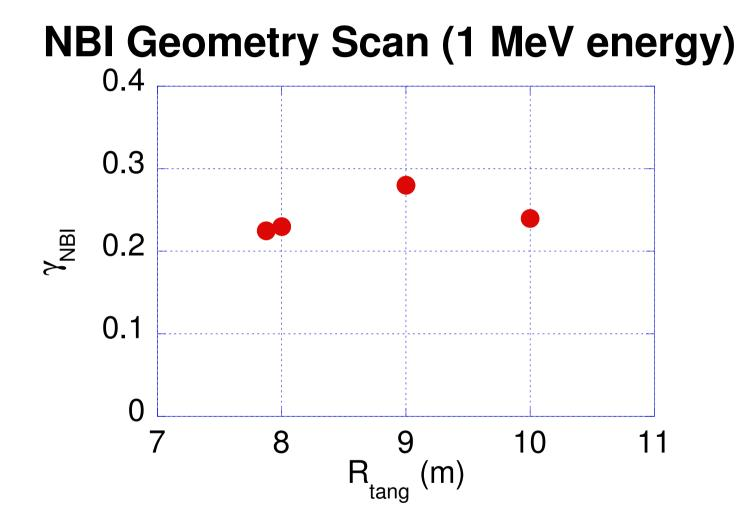
CD efficiency for different tangency radii, 1 MeV energy case. 1.5 MeV case investigated as well.
