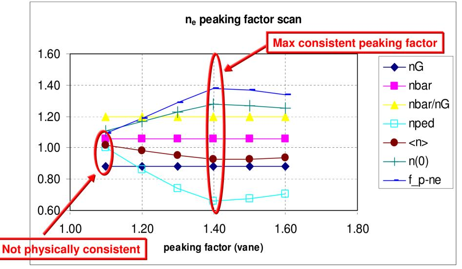
Working at fixed  $n/n_G=1.2$ , a density peaking of 1.4 is the most consistent choice (scan performed at fixed pedestal pressure).
