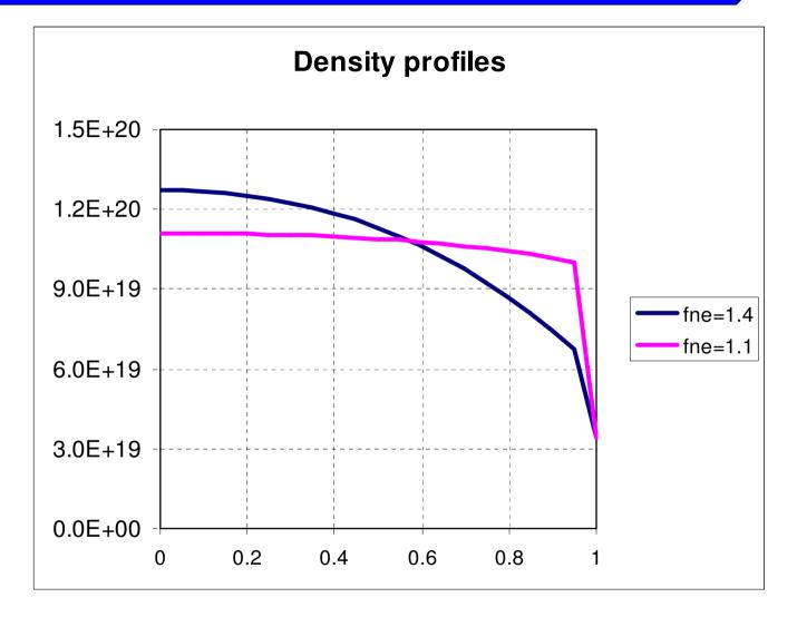
Resulting density profiles for 2 different peaking factors. Note that a density peaking factor of 1.1 leads to a pedestal density larger than  $n_G$  and is though to be not realistic.
