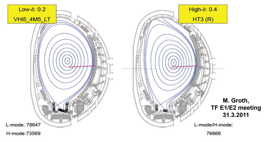
Strike point sweeps (± 2cm) are needed in all discharges to get good profiles from Langmuir probe and W influx measurements
